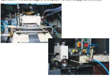
amount of lubricant required for any particular operation. This eliminates the mess and waste associated with in-die spray systems and externally lubricated roller systems. By applying the proper amount of lubricant, there is little cleanup required and no recirculating coolants to treat or dispose. This means a Cleaner shop and less overhead, not to mention the savings due to reduced tool wear, improved part quality, and increased production rates.
