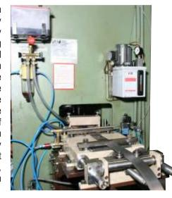
JSM Coil Stock Lubrication Systems are designed in modular way and have similar features between smallest unit to largest units. Due to modular design sizes uptill 1800mm can be build irrespective of material, speed, thickness. They are available in 3 basic models.
